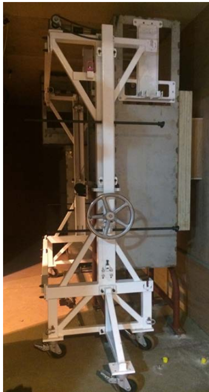
Fig. 2 – Trial of cabinet handling frame
