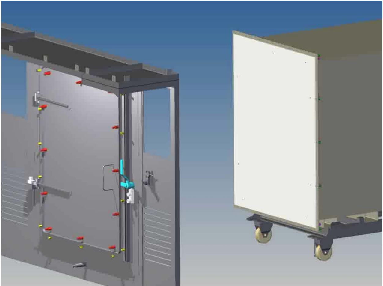
Fig. 3 – Schematic of crate export facility and crate liner
